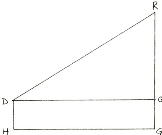
1. Segment RG represents the object you are going to measure. Point D is the location of your eye when you position the hypsometer. Point H is the location of your feet.
